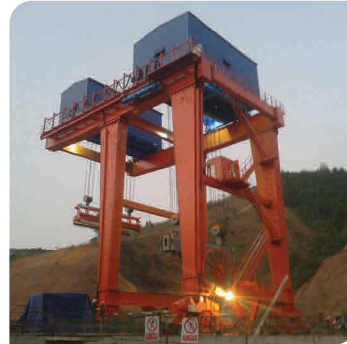
VINH HA HYDROPOWER PLANT - LIFTING CAPACITY: 2X100T/ 2X32T - SPAN: 8.5M - LIFTING HEIGHT: 40M - WORKING DUTY: 1AM
