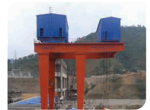
VINH HA HYDROPOWER PLANT - LIFTING CAPACITY: 2X100T/ 2X32T - SPAN: 8.5M - LIFTING HEIGHT: 40M - WORKING DUTY: 1AM
