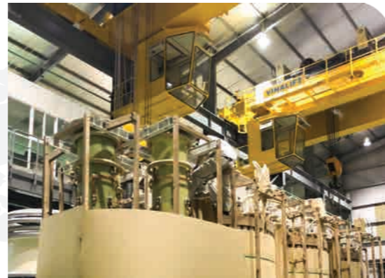
OVERHEAD CRANE - Lifting capacity: 100 Ton, 80 Ton
