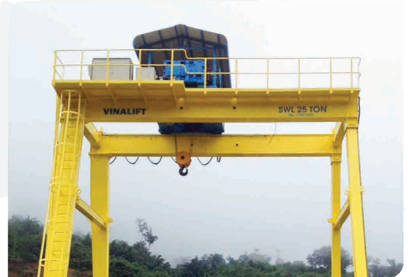
HYDRO POWER PLANT | GANTRY CRANE - Lifting capacity: 25T - Span: 9m - Lifting height: 50m
