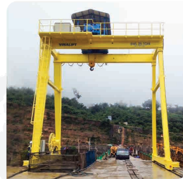
HYDRO POWER PLANT | GANTRY CRANE - Lifting capacity: 25T - Span: 9m - Lifting height: 50m
