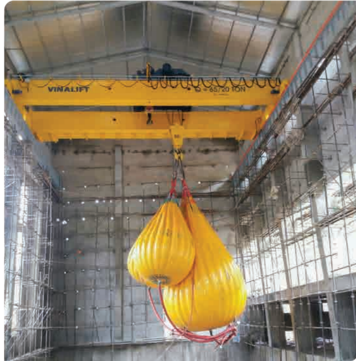
HYDRO POWER PLANT (NAM XAY) PORTAL CRANE - Lifting capacity: 65/20T - Span: 14.35m - Lifting height: 12m
