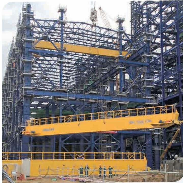
THERMAL POWER PLANT TURBINE HALL | OVERHEAD CRANE - Lifting capacity: 70/20T - Span: 30.5m - Lifting height: 35m.
