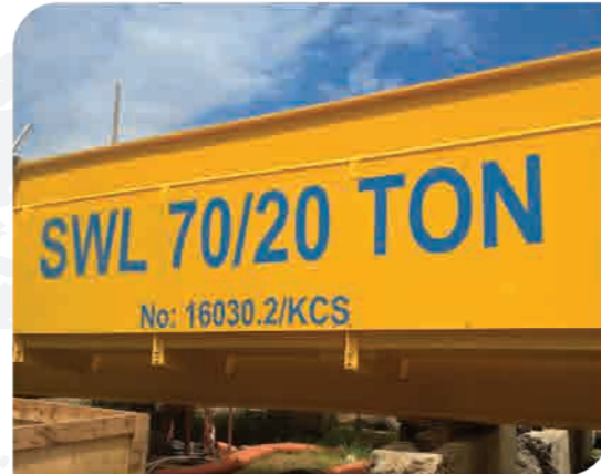
THERMAL POWER PLANT TURBINE HALL | OVERHEAD CRANE - Lifting capacity: 70/20T - Span: 30.5m - Lifting height: 35m.
