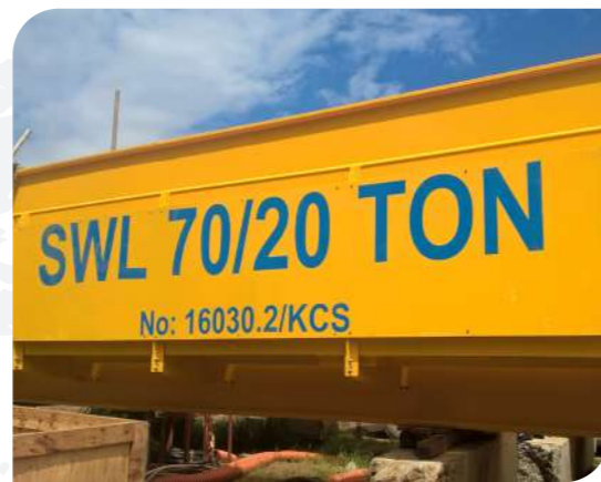
THERMAL POWER PLANT TURBINE HALL | OVERHEAD CRANE - Lifting capacity: 70/20T - Span: 30.5m - Lifting height: 35m.
