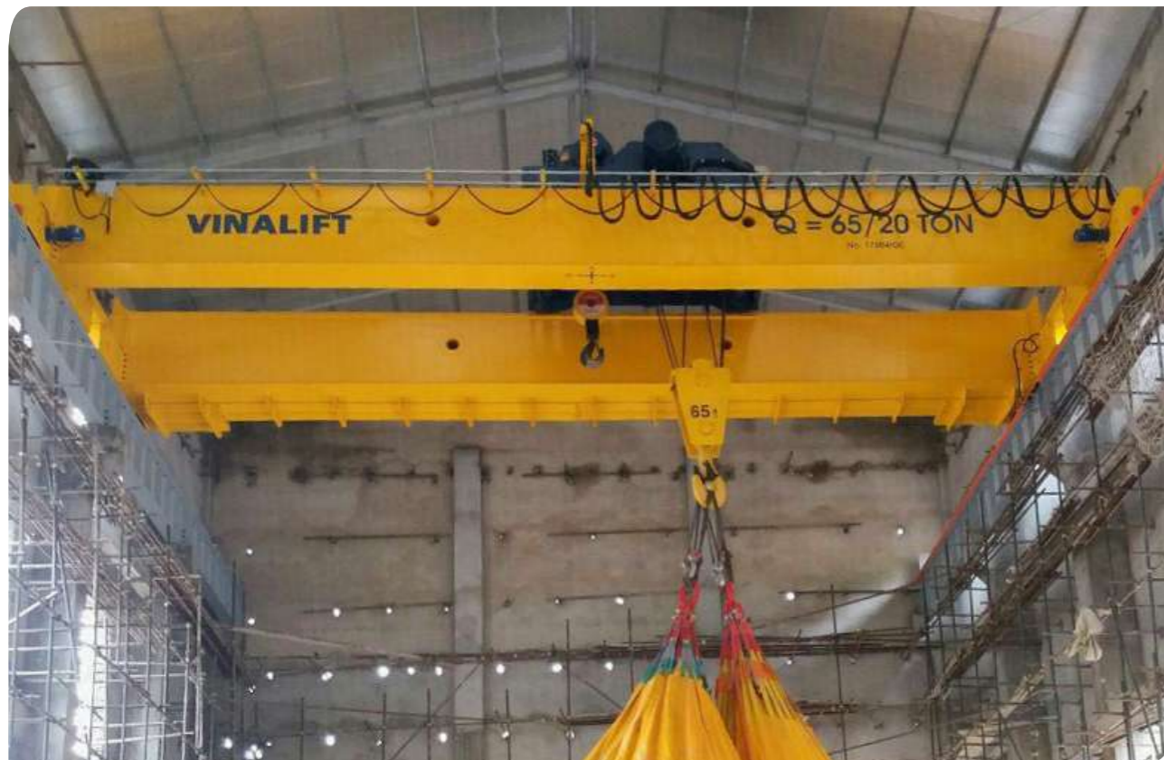
HYDRO POWER PLANT (NAM XAY) PORTAL CRANE - Lifting capacity: 65/20T - Span: 14.35m - Lifting height: 12m
